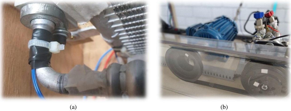
Figure 3. Temperature transducer (a) and compressor pulley-belt transmission system (b)
